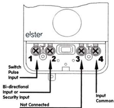
Note: Connections to reed-switch pulsers, such as AMCO Water Metering Systems' LRP (on the T3000) and T-probe for the V100 (red and blue wires), are made to pins 1 and 4. The security input requires a loop connection to the common input (between pin 2 and pin 4). A direction flag input is required for pin 2 and pulse input to pin 1 when used in a bi-directional mode.
