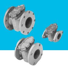
Operation. The strainer is a vertical Z-plate design to protect cold water meters from the damaging effects of debris and foreign matter. The strainer improves the velocity profile of the water being metered and minimizes the effects of velocity distortion caused by upstream valves and fittings. Consequently, the meter's accuracy is maximized by the elimination of debris and turbulence.
