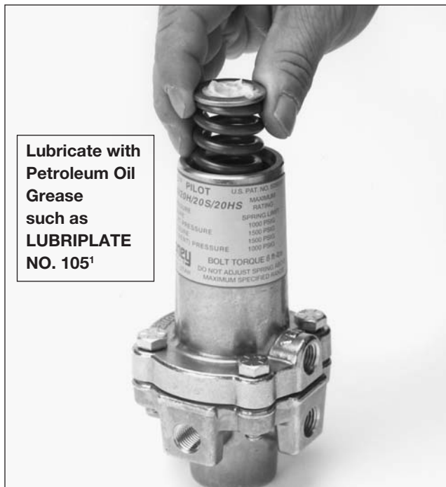
Figure 17 - Installing the Spring with lubricated Spring Follower.
