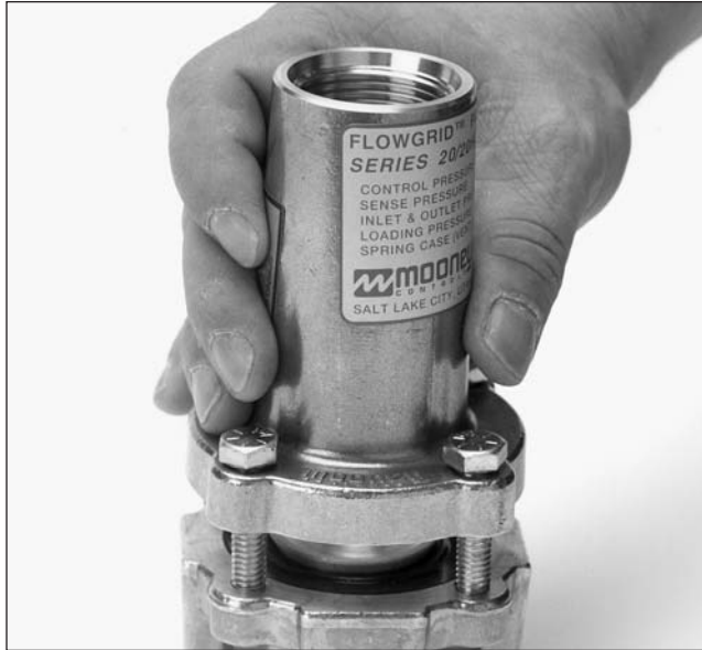
Figure 16 - Placing the Spring Housing on the Pilot Body.
