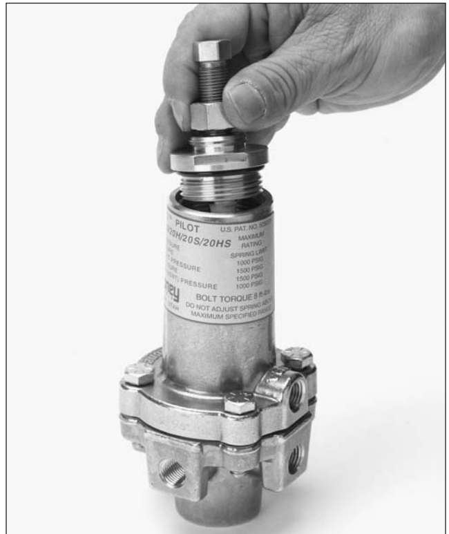
Figure 18 - Installing the closing cap assembly for Pilot with the Red, Cadmium, Blue, and Purple Springs.
