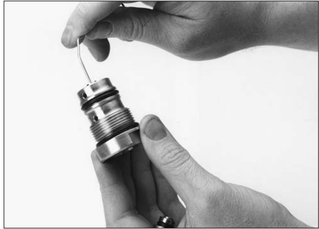
Figure 13 - The orifice can be pushed out of the Body Insert (Cartridge) using a paper clip.
