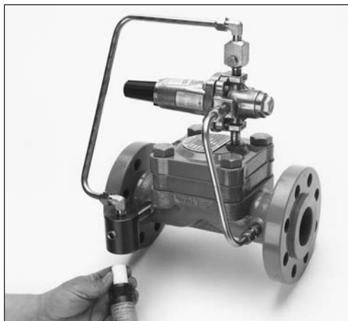
Figure 1 - The Type 30A Mooney® Filter with Filter Housing removed allowing easy inspection of the element. Mounted on a 2" large single Port Flowgrid® Regulator with Series 20 Pilot and Type 24 Restrictor.
