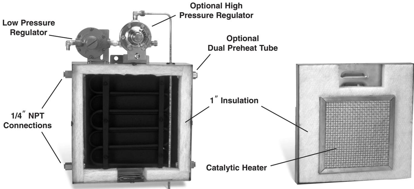
Supply to the preheat tube in/out connection is facilitated with rigid hex head 1/4" NPT female, bulkhead outlets located on the side of the heater. A dual preheat tube is optional.
