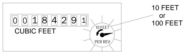
This index would be mounted on a 10 foot drive meter as indicated by the 10 on the sweep hand. This reading is 0184291 SCF if you bill in hundreds CCF your reading would be 01842 if you bill in thousands MCF your reading would be 0184
