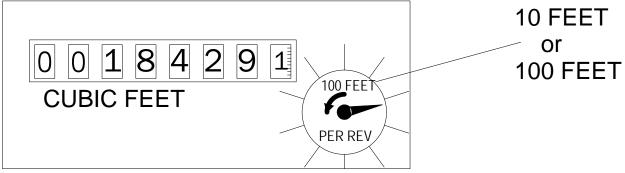
If this index is mounted on a 100 foot drive meter and has a 100 on the sweep hand. This reading is 0184291 0 SCF
